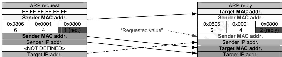
Figure 2.9. Memory swapping between ARP request and reply packets
