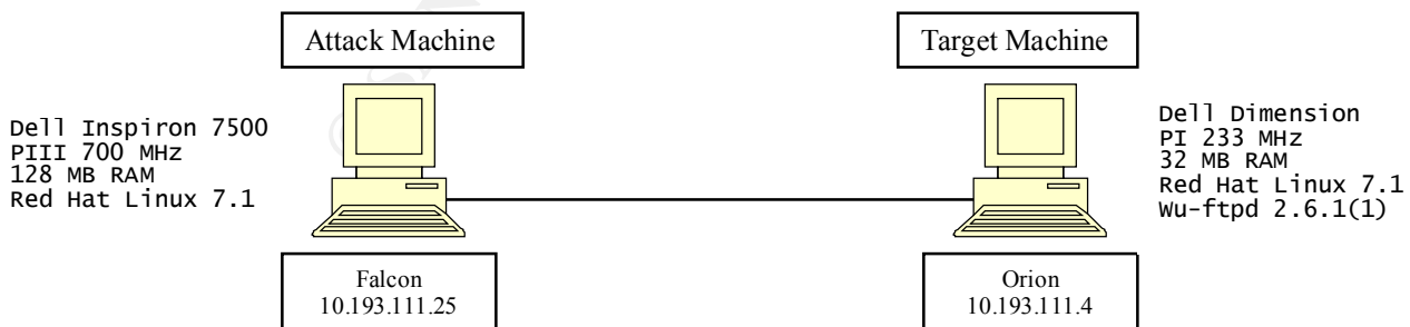
Figure 2.12: Test Network Configuration
