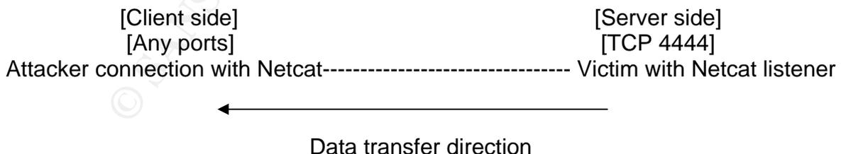
From the ethereal, it shows the attacker with port 1033 connected to port 4444 on the victim.
