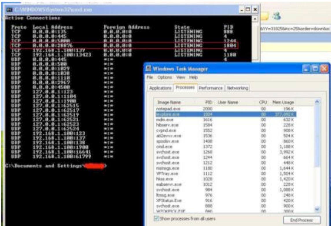
It has been established that Internet Explorer with process ID 1804 is listening on TCP port 28876. To see if there is a Windows command shell there, it is necessary to connect to the port.
