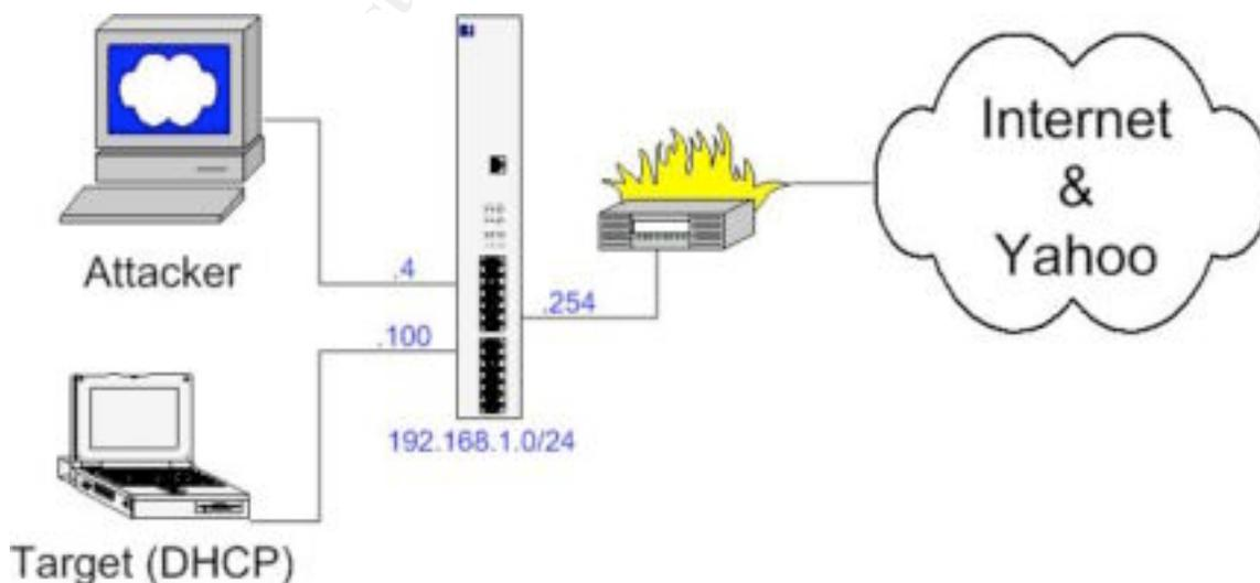
The target machine, labeled "Target" in the network diagram is a Windows XP Service Pack 1 laptop. The target machine has all patches applied, except MS04-040. The patch was released while the lab environment was being built and configured. The target machine is also running Symantec Anti-Virus Corporate Edition (SAV-CE) version 8.1 and is using the 11/29/2004 rev9 virus definitions. For these experiments, a local user was added and configured and placed in the Administrators group.
